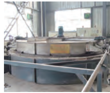
6m Tempering Equipment
