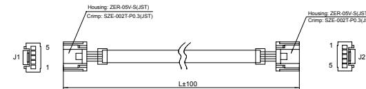
◇ RS-232 Communication Cable(P/S/Q Type)(TSM23/24/34)
