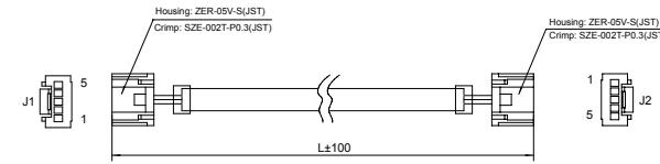
◇ RS-232 Communication Cable(C Type)(TSM17/23/24/34)
